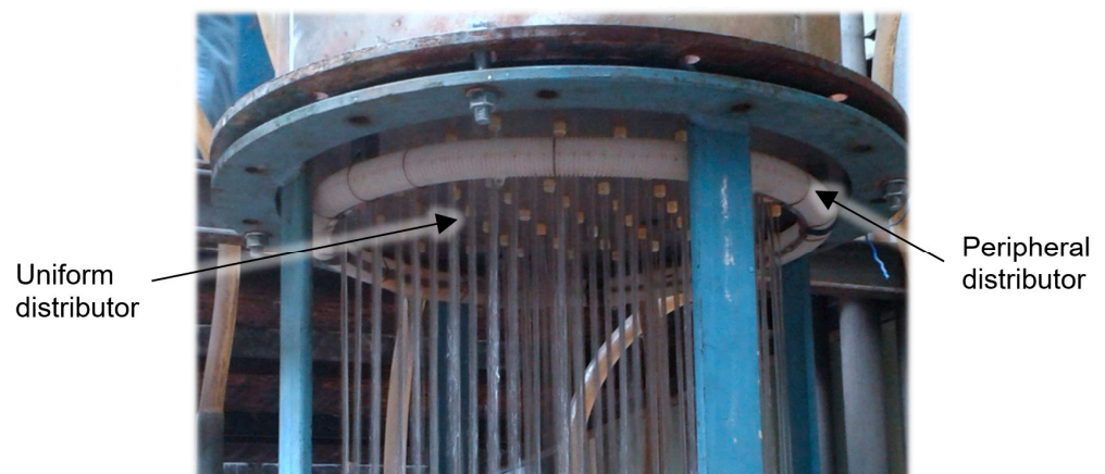
Figure 3. Photography of the uniform distributor operation.
