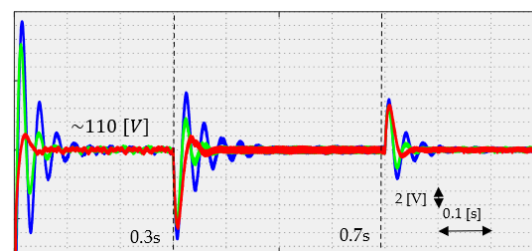
Figure 10. The waveforms of capacitor voltage of the FB DC-DC power converter under Scenario III (PI controller shown in blue, SMC controller shown in green, and proposed technique shown in red).
