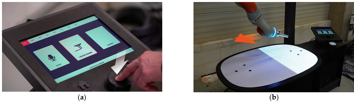
Figure 20. (a) Operator pushes rotary dial. (b) Cobot “pulls” images out of display and spreads them across work surface.
