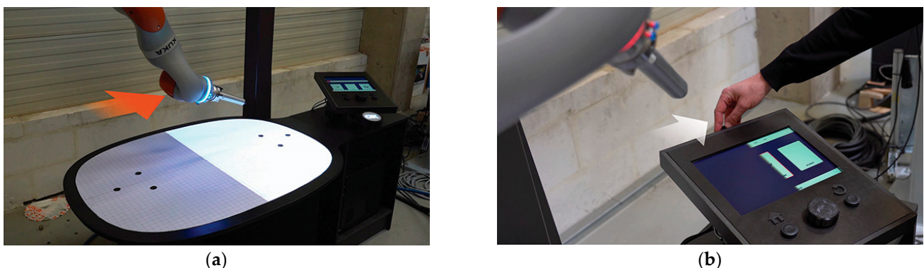
Figure 26. (a) Cobot moves towards the control unit, takes projection with it, and “pushes” images in display. (b) Operator deactivates system by moving slider to right.
