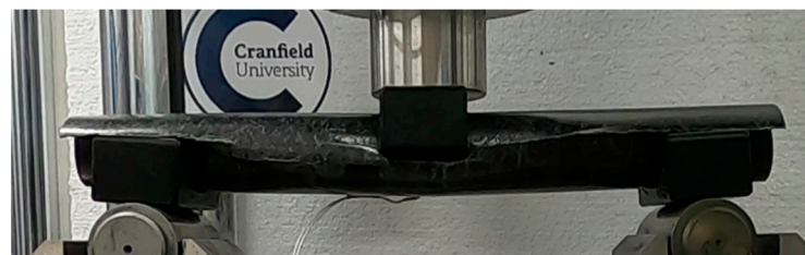
Figure 3. Typical failure mode observed during the three-point bend tests (OD58-1).
