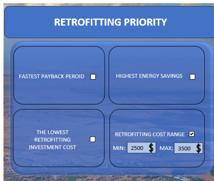
Figure 18. The third section of the EERMGCs tool input tab, where the user determines their objective and priorities in choosing the energy retrofitting measures.
