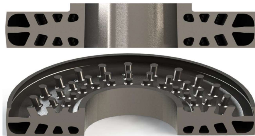
Figure 10. Rendered CAD model of the optimised geometry of the rotoric component (diametral section and 3D rendering of half collar) [20].
