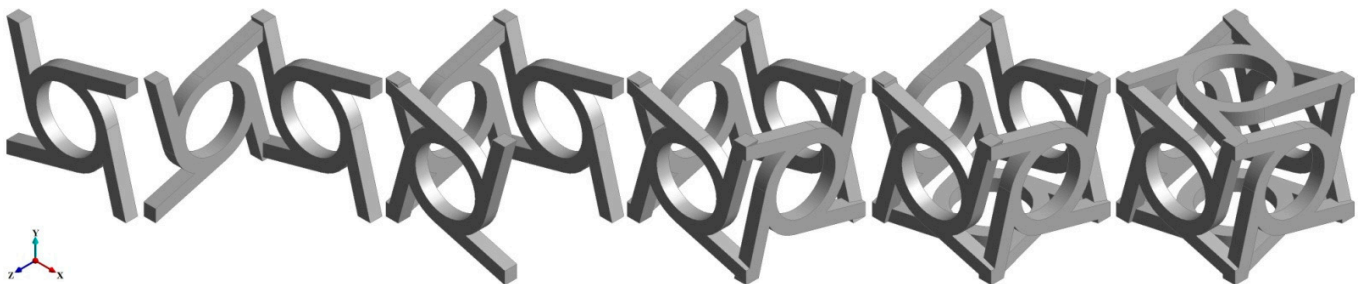
Figure 2. Formation of a metamaterial unit cell.
