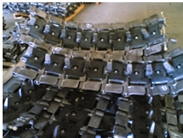
Figure 5. Assembled track segments.
