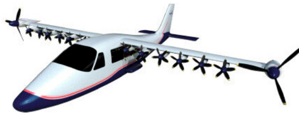
Figure 32. Sketch of the flight test demonstrator of SCEPTOR project. Image adapted from [166].
