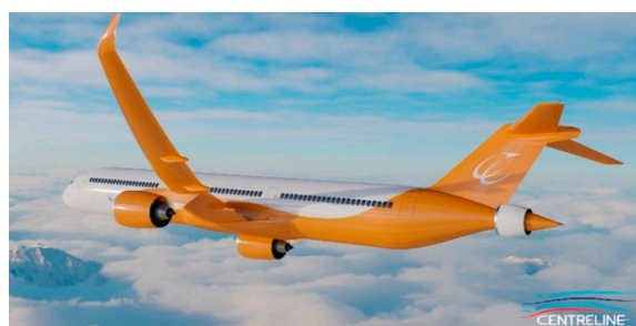
Figure 55. CENTRELINE turbopropulsive fuselage concept. Image adapted from [209].
