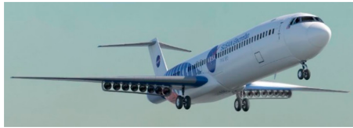
Figure 44. Representation of SUSAN transport aircraft concept. Image adapted from [179].
