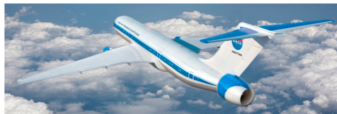
Figure 56. NASA STARC-ABL concept, as described by Welstead and Felder [219].
