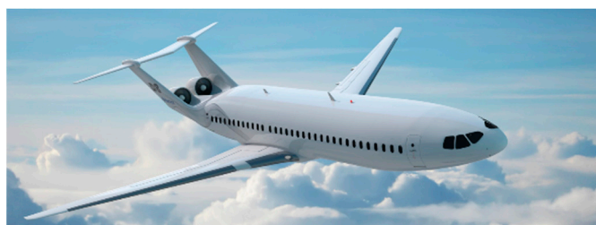
Figure 58. The Double Bubble D8 concept, as presented by Drela [110].
