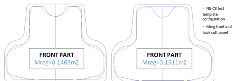
Figure 12. Comparison of Version 3 M regular-sized soft panel configuration with the equivalent NIJ-C3 test template [6] (developed in CAD Grafis).
