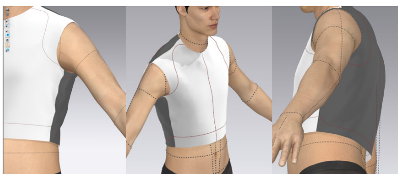
Figure 15. Virtual fitting of the BPSP patterns for M regular size in the Clo3D program.
