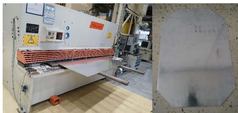
**Figure 16.** The blank cutting in progress (left) and the resulting blank (right).
