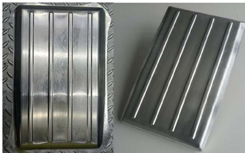
**Figure 18.** The deep-drawn monolithic rooftop tent, before trimming (left) and after trimming (right).
