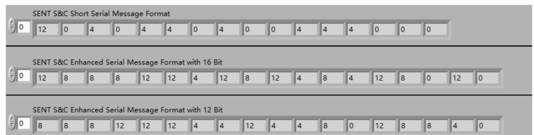
Figure 9. Status pulse values in serial message format.
