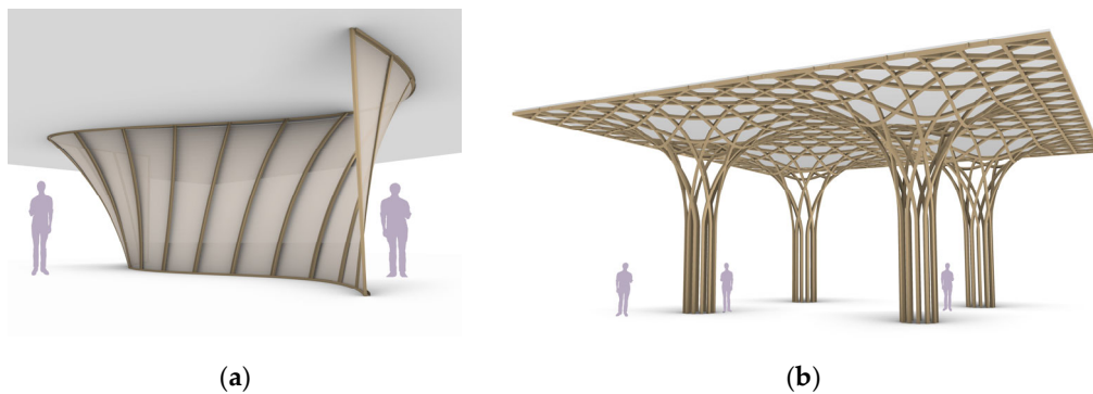
Figure 10. Speculation on the possible use of customised NFRP profiles: (a) as a hidden substructure giving shape to a partition wall, further covered with formable panels (balsa boards, gypsum boards, textiles, and other NFRP panel products); (b) as a free-formed framework from customised NFRP profiles.
