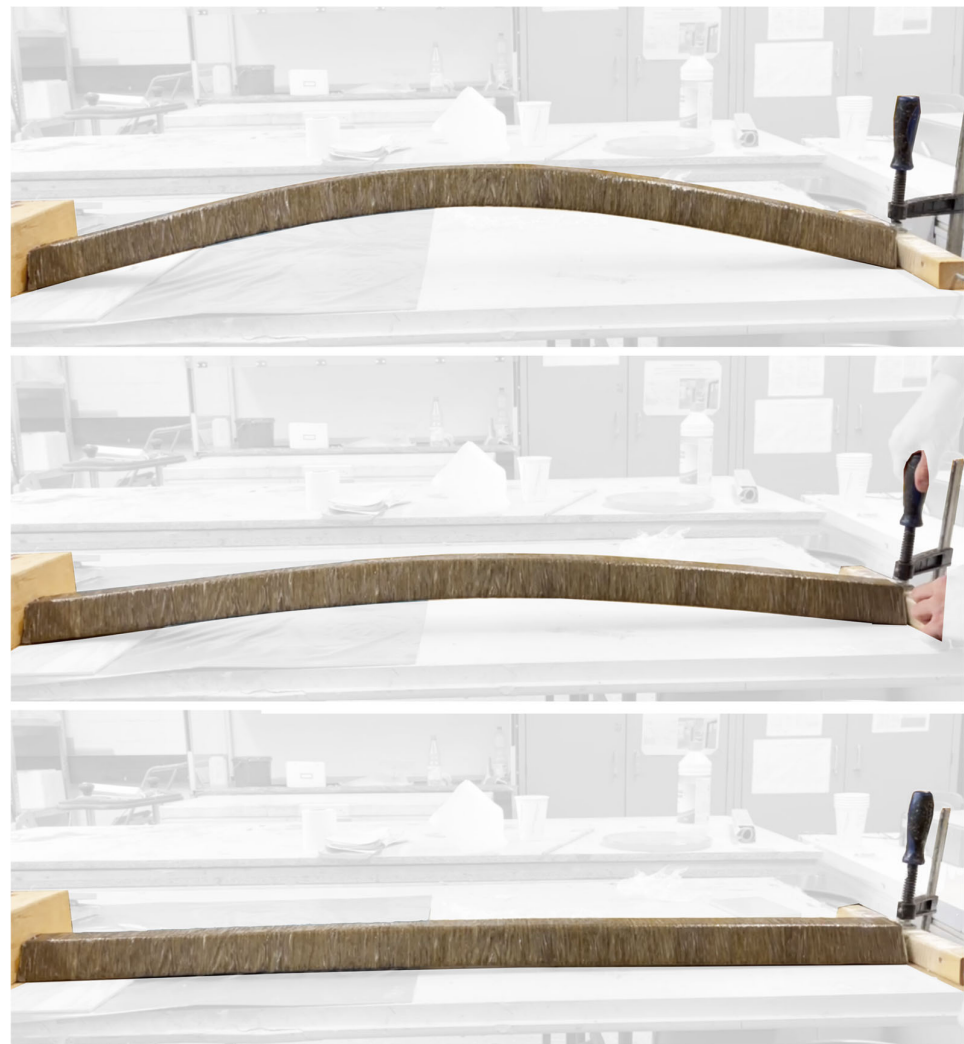
Figure 1. A cured profile with a winding angle close to 90^\circ snaps back to its original straight shape immediately after being released (frames taken within 3 s).
