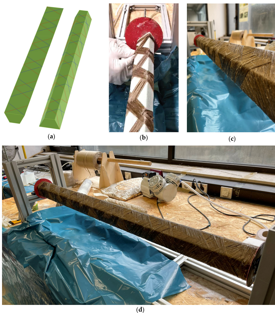
Figure 2. (a) Preview of a winding path, later sketched on the core to support the manual winding process; (b) Binding process in progress; (c) Winding pattern at 50° angle; (d) Accomplished winding process, before the forming stage.
