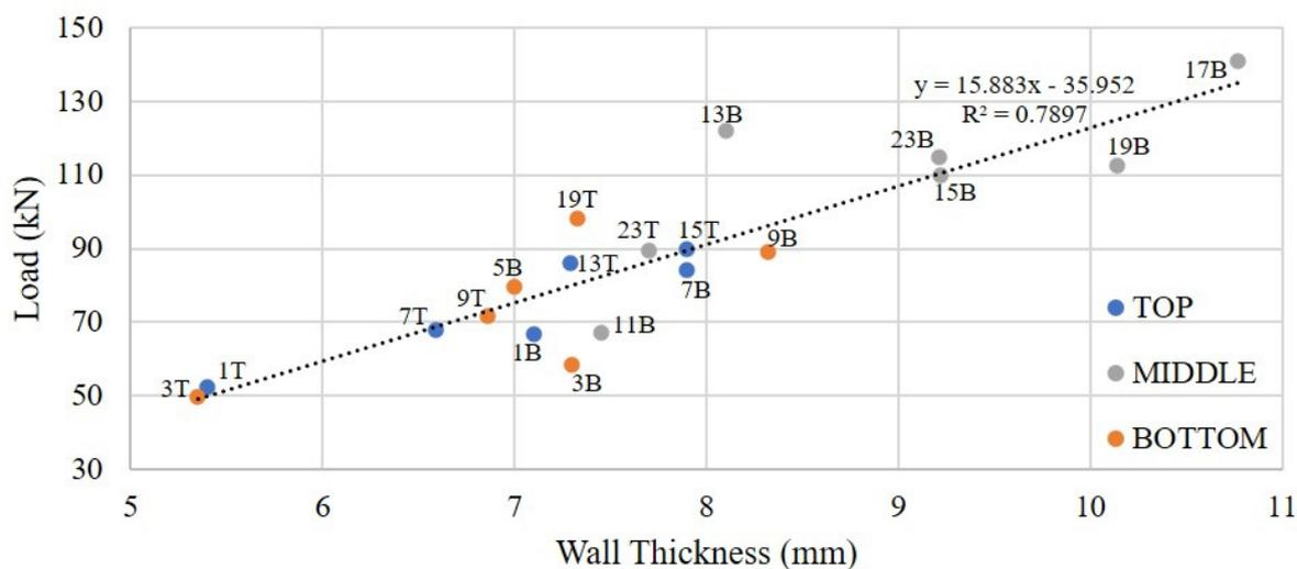
**Figure 10.** Influence of node location with respect to wall thickness (mm) and compressive load (kN).
