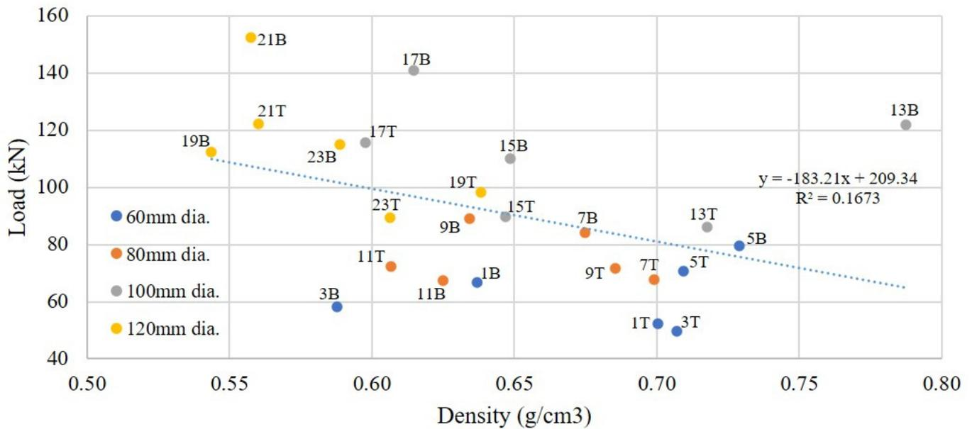
Figure 5. Density vs. the compressive load capacity with respect to culm diameter.
