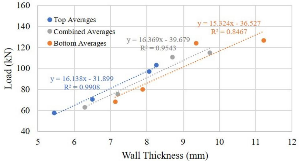
**Figure 7.** Average wall thickness vs. average maximum compressive parallel-to-grain load, with respect to bamboo culm diameter and consideration to top and bottom representatives.
