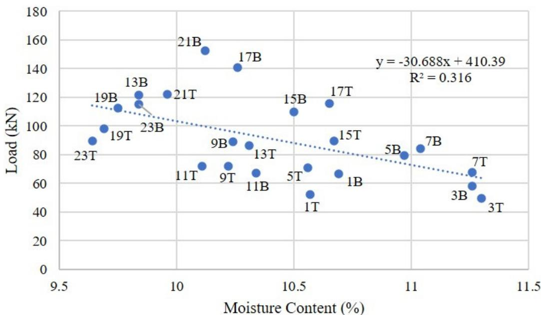
Figure 4. Moisture content vs. compressive load capacity.
