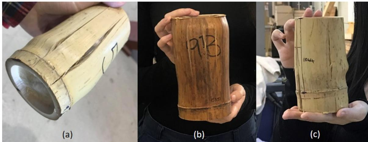
**Figure 11.** Post-compression failure of representatives (a) 5B (b) 9B (c) 9T.
