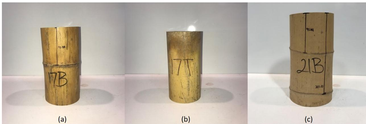
**Figure 2.** Examples of representatives prior to compression testing with a distance of a node from the top (a) 17B—one node (b) 17T—no node (c) 21B—two nodes.
