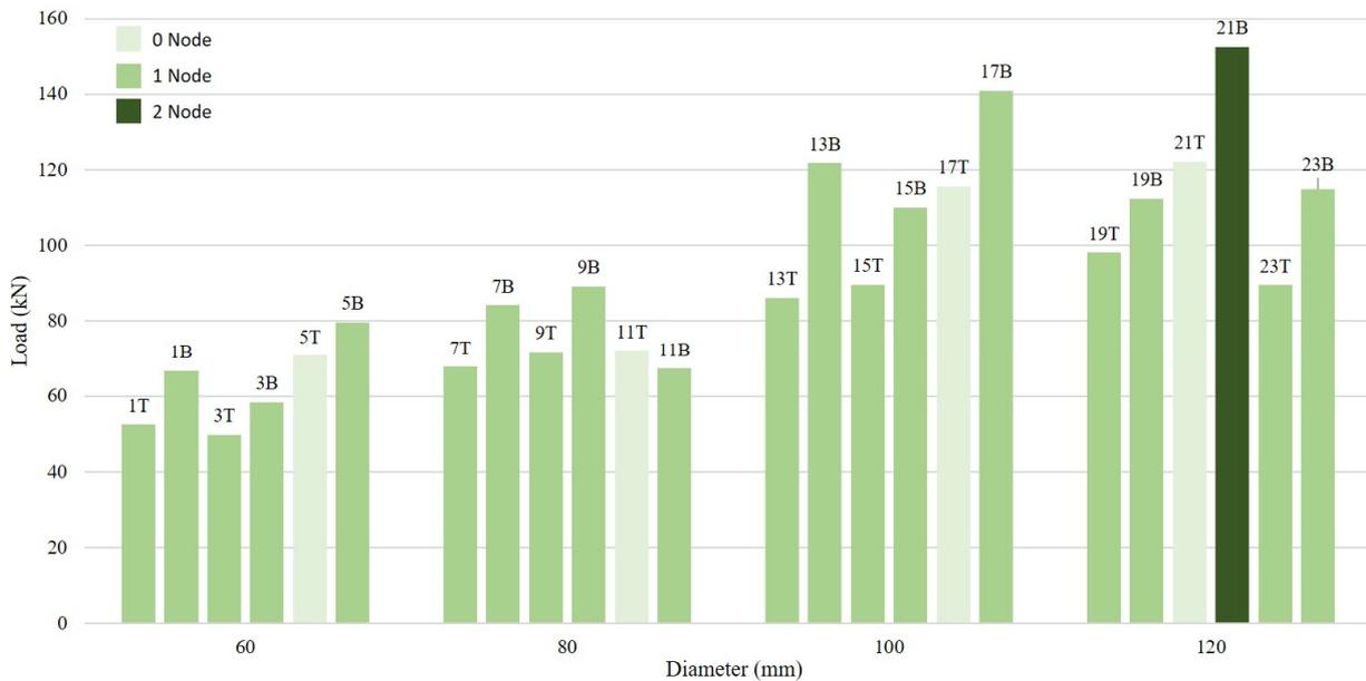
**Figure 8.** Ultimate load capacity by diameter with respect to the number of nodes.
