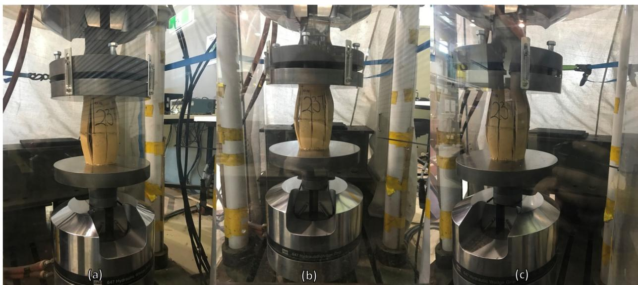
**Figure 3.** UTM testing final deformation of representative 23T (a) left side profile (b) front profile (c) right side profile (Note: protective sheeting and Plexiglas around testing setup to allow for safer controlled failure).
