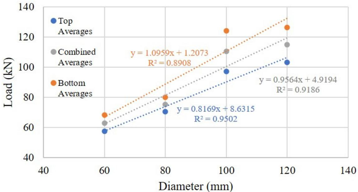
Figure 9. Diameter vs. average load capacity with consideration to top and bottom representatives.
