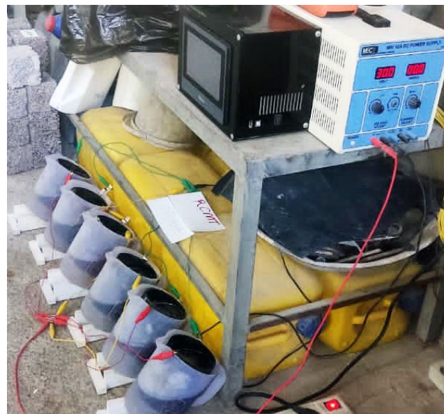
Figure 5. Rapid Chloride Migration Test (RCMT).
