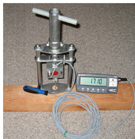
Figure 13. Screw withdrawal force meter (Designed by Fakopp Enterprise Bt., Hungary).
