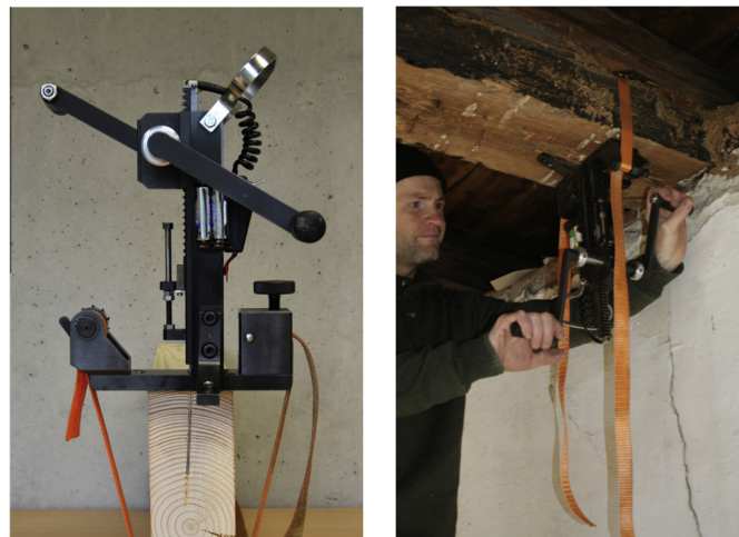
Figure 14. The pin-pushing device used for in situ testing (Courtesy of Kloiber et al. [44]).
