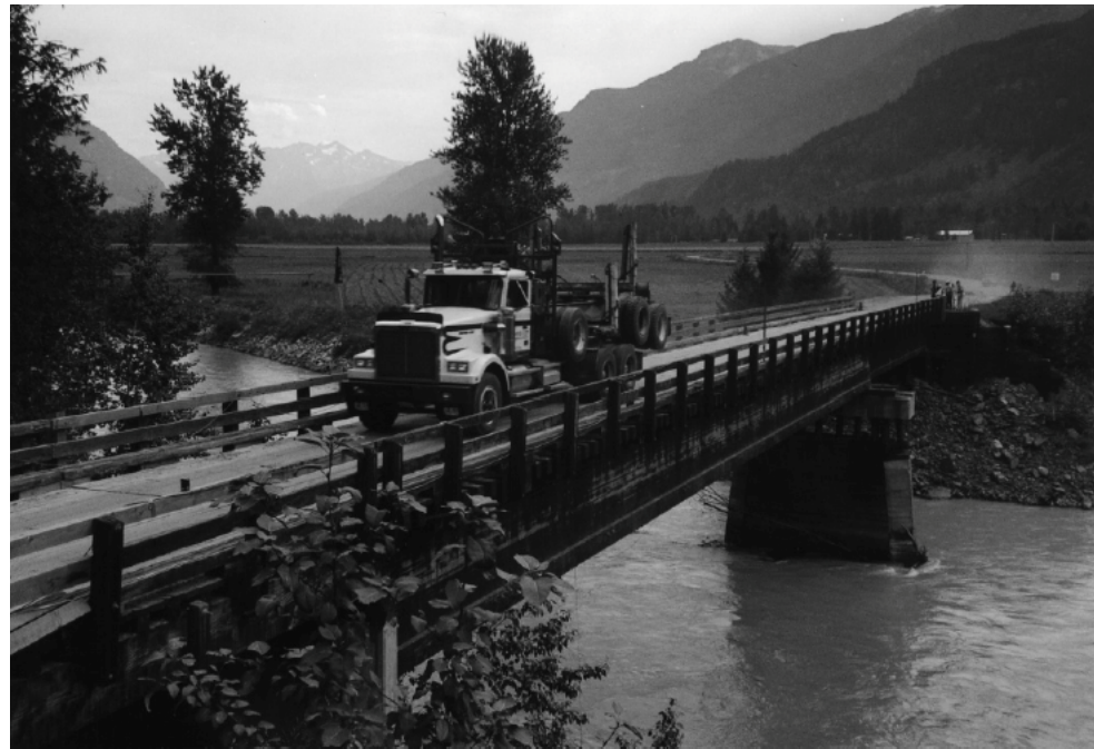
Figure 8. Forced vibration testing with truck passing over long span bridge (Courtesy of Horyna et al. [35]).
