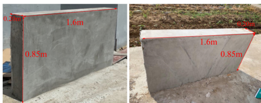
Figure 8. The wall sample built to be used in the context of estimating the severity of damage (crack depth) in a wall [58].
