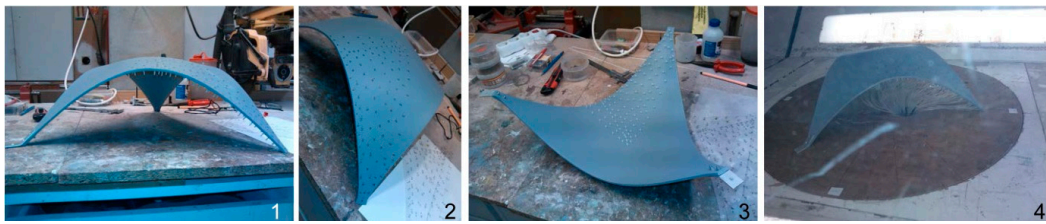
Figure 12. Final scale model: (1–3) different views of the final scale model; (4) preliminary tests at the closed circuit aerodynamic tunnel at LNEC.
