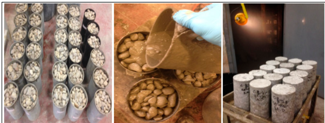
Figure 2. TSC specimen preparation showing preplaced aggregates in cylindrical molds (left), placement of grout by gravity (center) and final demolded specimens (right).
