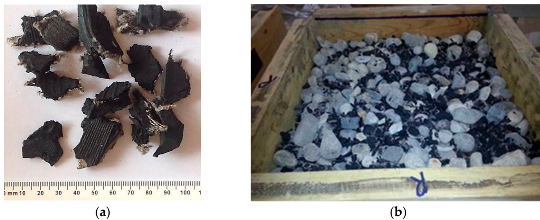
Figure 3. Overview of (a) tire rubber particles, and (b) preplaced RCA with scrap tire rubber granules and steel wire.
