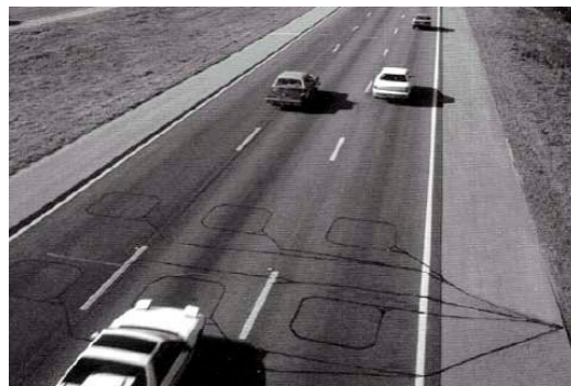
Figure 5. Induction loop detectors at freeway location on the roadway [16].
