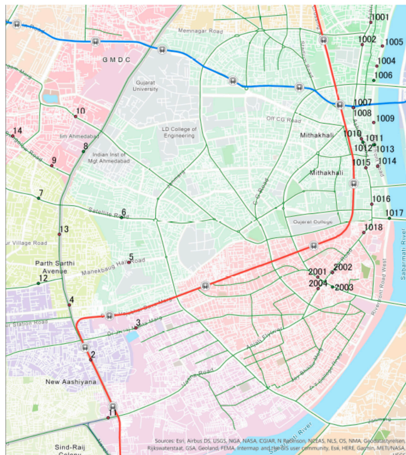
Figure 4. Traffic measurement environment in Ahmedabad city (the number is defined each CCTV installed location. Blue line and red line are the Metro line which is under development).
