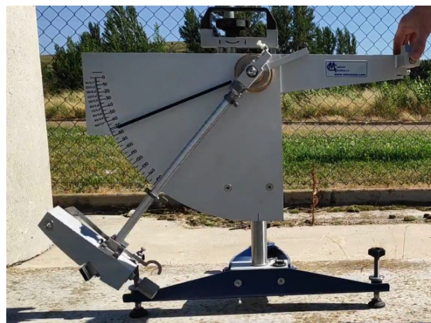
Figure 10. Friction pendulum (TRRL pendulum).
