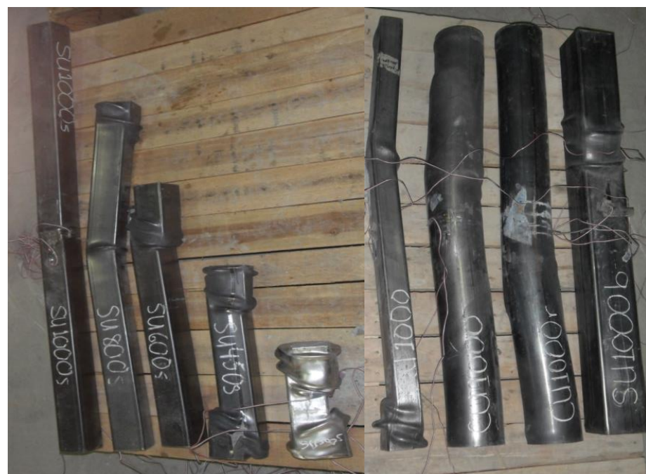
Figure 5. Failure modes of UHSC-filled CFST columns (from left: Us2-20, Us2-16, Us2-12, Us2-9, Us2-6, Ur-20, Ucl-9, Ucl-9, and Us4-10).
