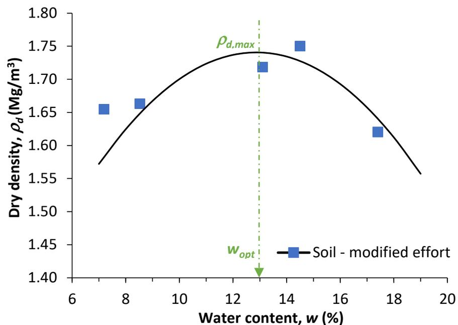
Figure 4. Proctor test results of soil with modified compaction effort.
