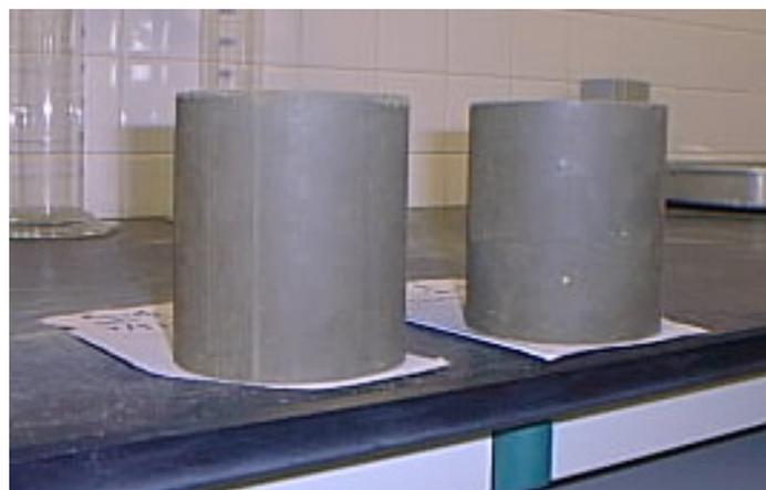
**Figure 6.** Cement-bound soil specimens.
