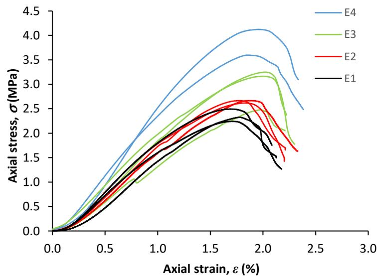
Figure 8. UCT stress–strain curves for CBS specimens with 14% cement.
