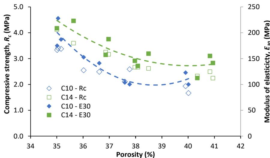
Figure 9. Effect of porosity on unconfined compressive strength and modulus of elasticity.
