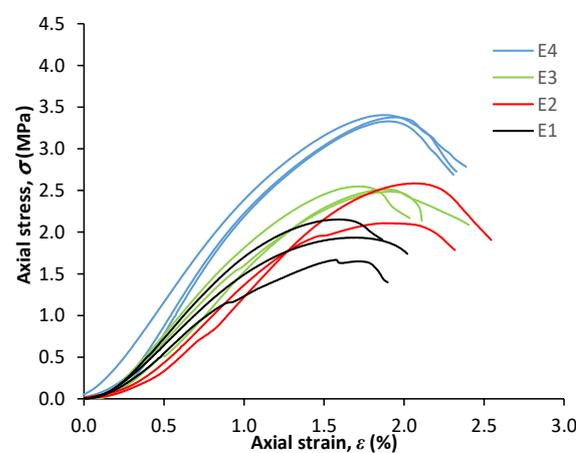
**Figure 7.** UCT stress–strain curves for CBS specimens with 10% cement.
