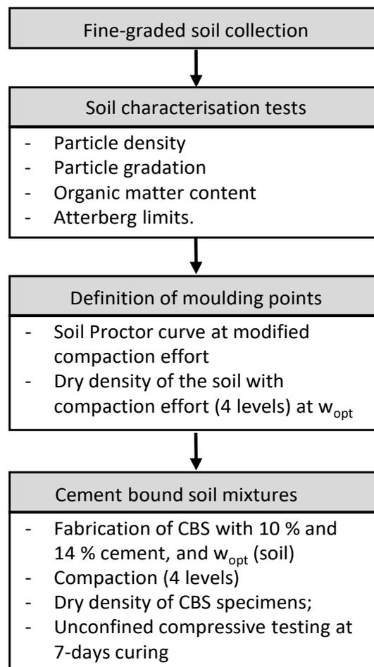
Figure 1. Diagram of the experimental plan.
