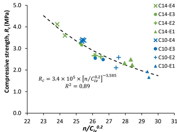
**Figure 11.** Effect of modified ratio of porosity to volumetric cement content on unconfined compressive strength.
