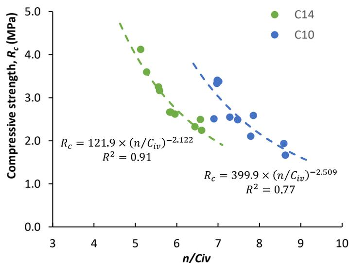
Figure 10. Effect of the ratio of porosity to volumetric cement content on unconfined compressive strength.
