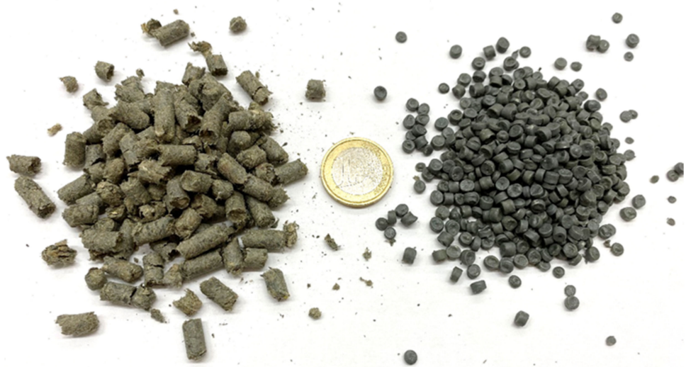
Figure 4. The cellulose-synthetic fiber containing plastomeric polymers vs. plastomeric polymer compound. The scale coin is EUR 1; 23.25 mm.
