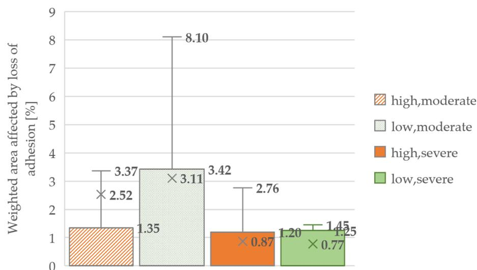
Figure 7. Boxplots of the weighted area of the façade affected by loss of adhesion anomalies according to the buildings’ height and exposure to wind–rain action.
