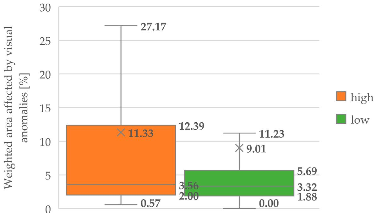
**Figure 3.** Boxplots of the weighted area of the façade affected by visual anomalies according to the buildings’ height.
