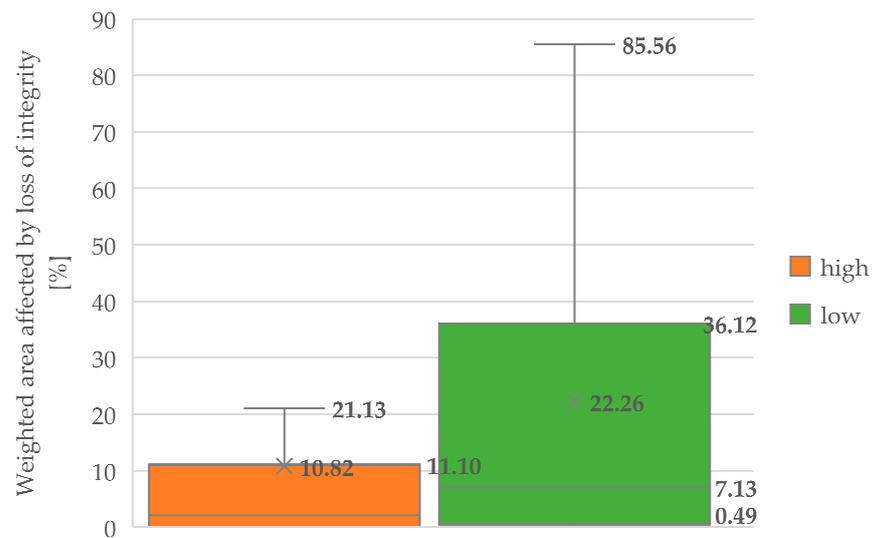
**Figure 5.** Boxplots of the weighted area of the façade affected by loss of integrity according to the buildings' height.
