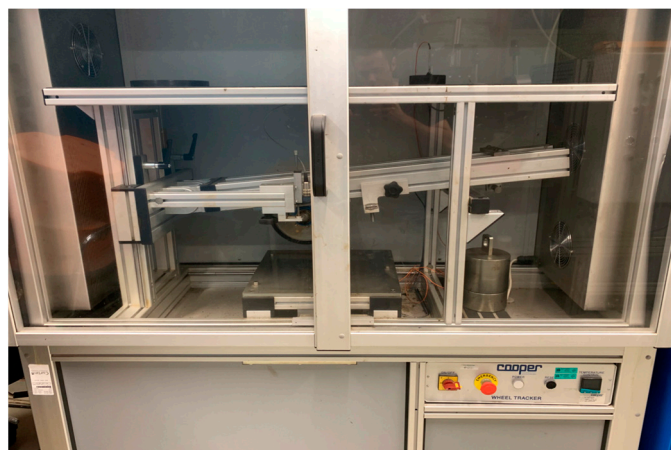
Figure 4. Cooper wheel tracker device.
