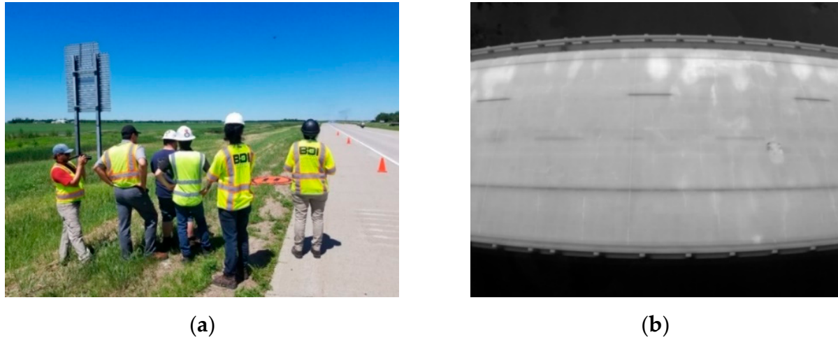
Figure 2. IRT data collection depicting (a) crew collecting data with a UAS and (b) sample of IRT image.
