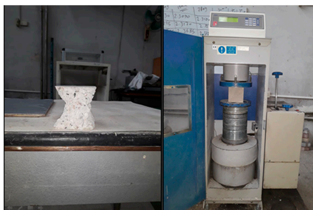
Figure 6. Compressive strength test.
