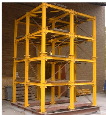
Figure 5. ASCE experimental SHM benchmark structure: experimental model (excerpt from [38]).
