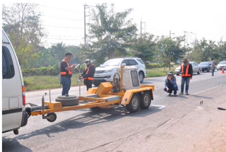
Figure 4. Dynatest Model 8000 falling weight deflectometer (FWD) from Denmark.
