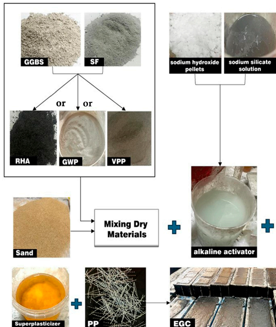
Figure 2. Materials and mixing method used in this study.
