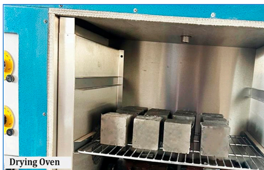
Figure 3. Heat curing of EGC specimens for 24 h after demolding.
