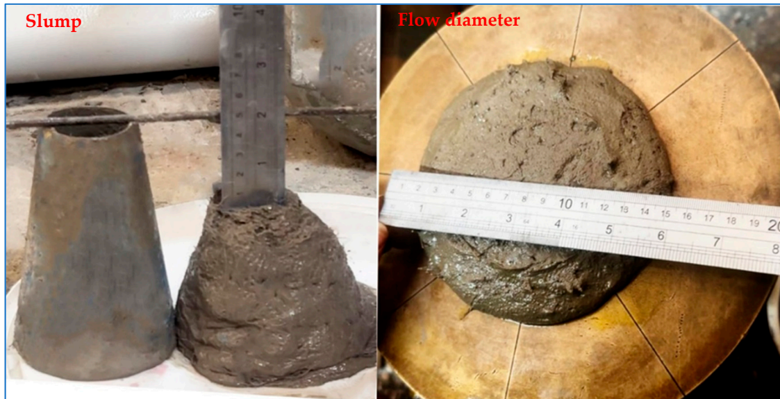
Figure 4. Measuring of EGC workability.
