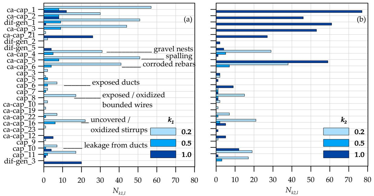
**Figure 8.** Number of defects detected on PC girders of bridges of highway A18 at different (a) extension and (b) intensity grades.
