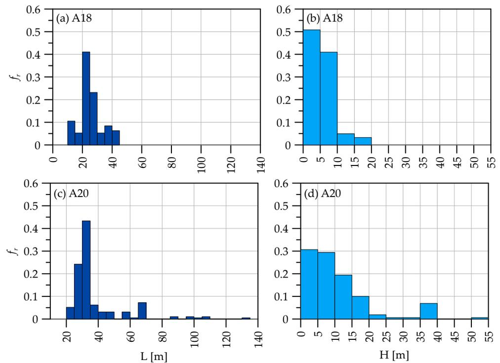
**Figure 4.** Relative frequency ( $f_r$ ) of length of girders ( $L$ ) and maximum height of piers ( $H$ ).
