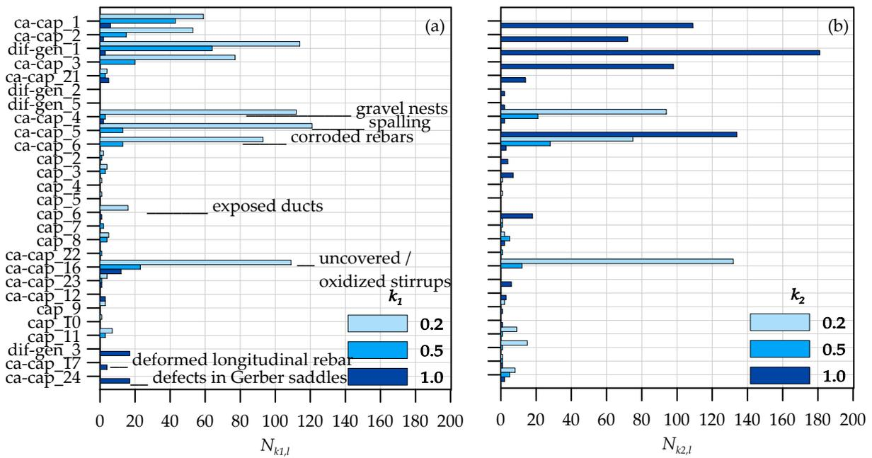
**Figure 9.** Number of defects detected on PC girders of bridges of highway A20 at different (a) extension and (b) intensity grades.
