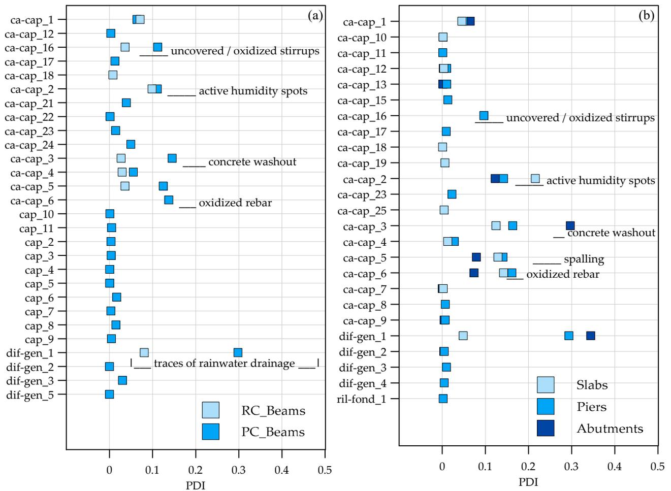
**Figure 12.** Prioritization defect index for PC bridges of highway A20: (a) PC girders and RC beams, (b) slabs, piers and abutments.
