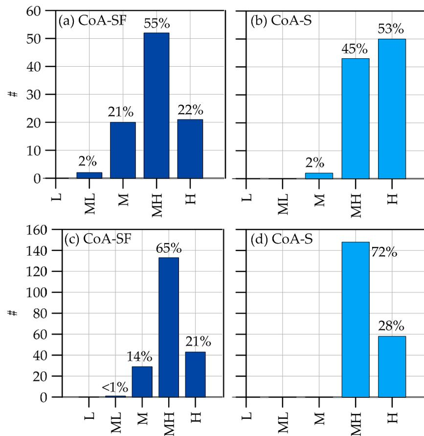
**Figure 10.** Structure–foundation (*SF*) and seismic (*S*) classes of attention of investigated PC bridges: (a,b) A18, (c,d) A20.
