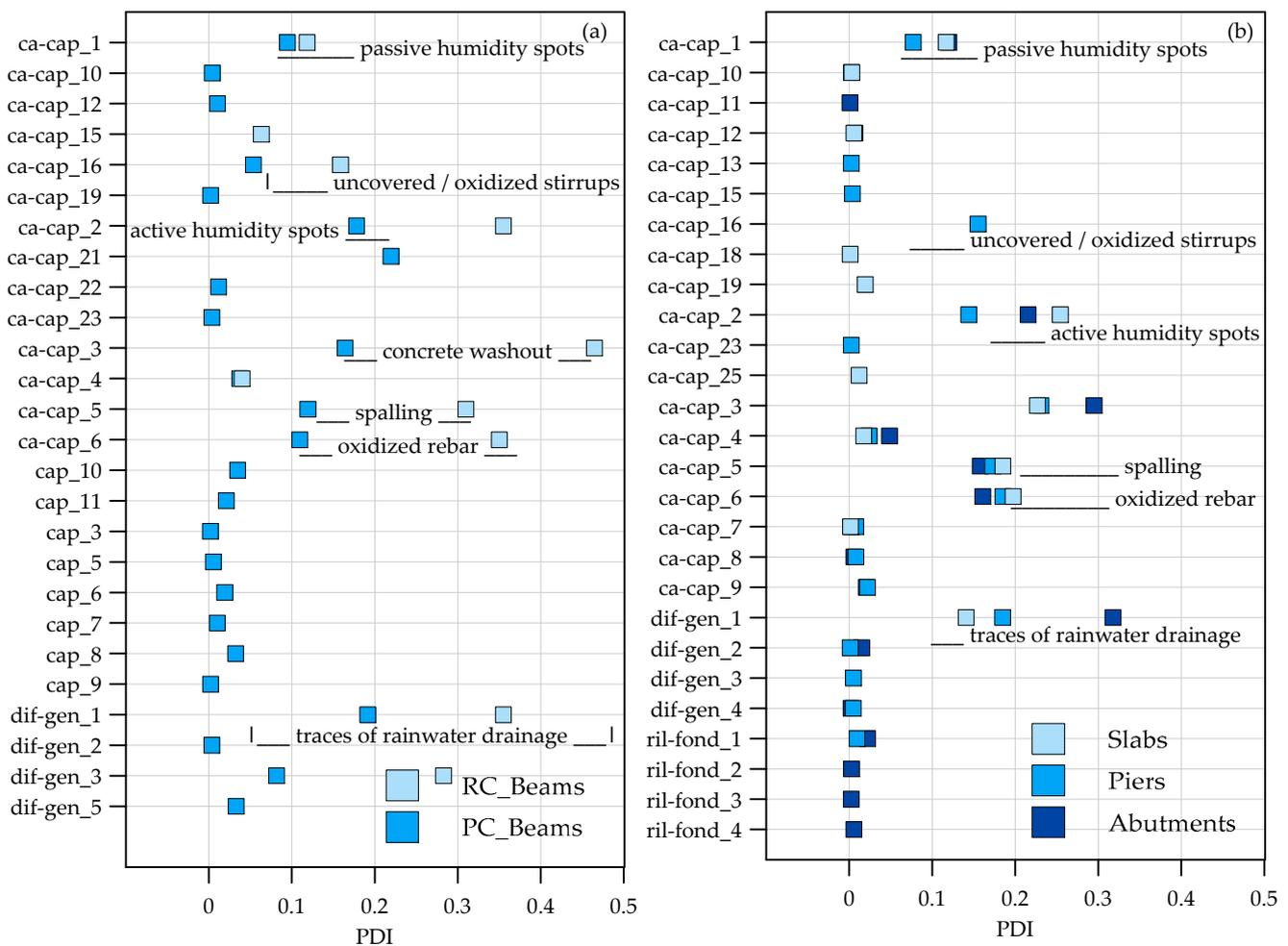
**Figure 11.** Prioritization defect index for PC bridges of highway A18: (a) PC girders and RC beams, (b) slabs, piers and abutments.
