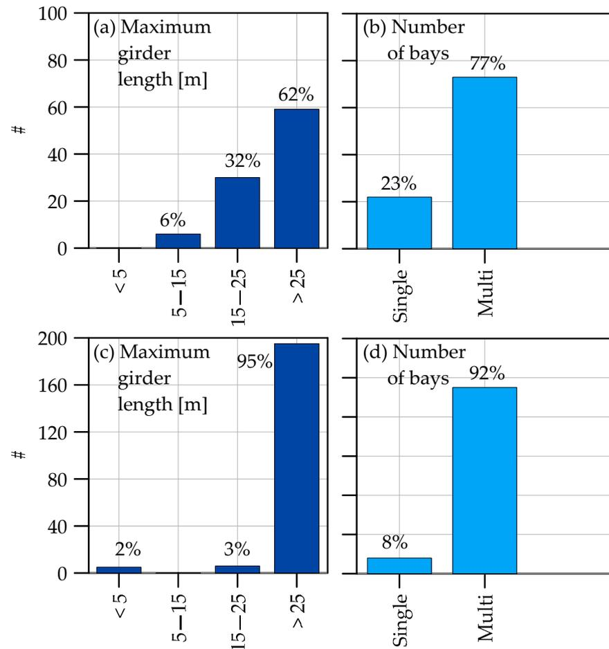
**Figure 5.** Maximum girder length and number of bays of the investigated PC bridges: (a,b) A18; (c,d) A20.
