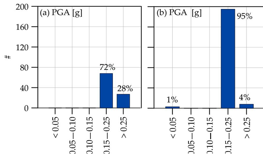
Figure 6. Peak ground acceleration at bedrock for the investigated PC bridges: (a) A18 and (b) A20.
