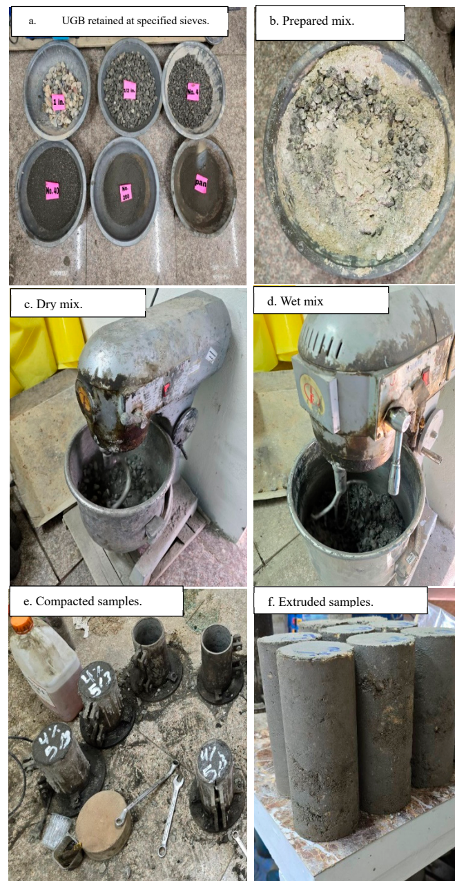
Figure 5. Sample preparation sequence. (a) UGB retained at specified sieves, (b) prepared mix, (c) dry mix, (d) wet mix, (e) compacted samples, and (f) extruded samples.
