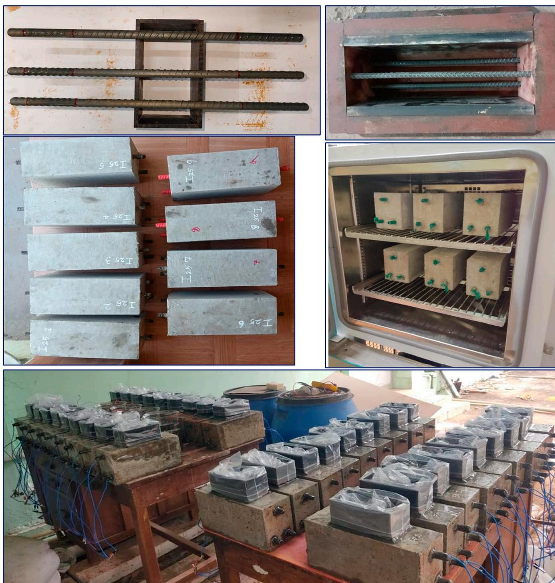
**Figure 4.** Stages of Macrocell Corrosion Testing Setup for Concrete Specimens.
