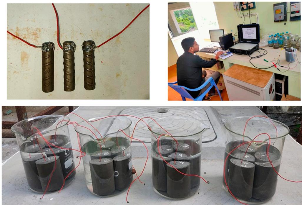
**Figure 5.** Electrochemical Testing Setup for Corrosion Evaluation.
