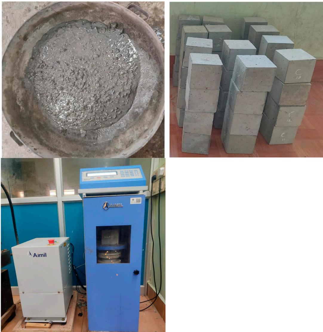
**Figure 3.** Preparation, casting, and compressive strength testing of concrete specimens.
