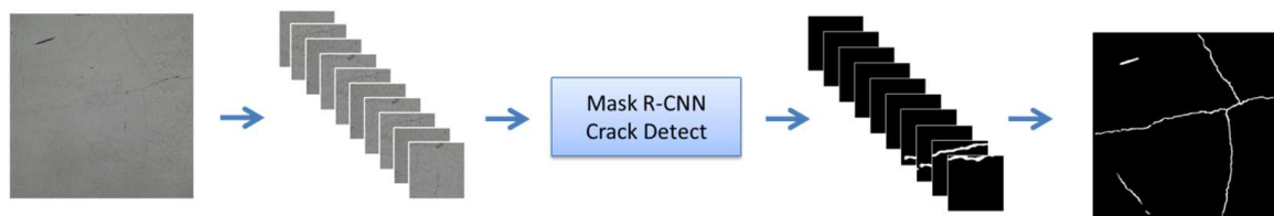
Figure 3. Flowchart of the process for generating crack masks: The original image is segmented, and the cracks are recognized using the Mask R-CNN model. The results are then stitched back to the original size.
