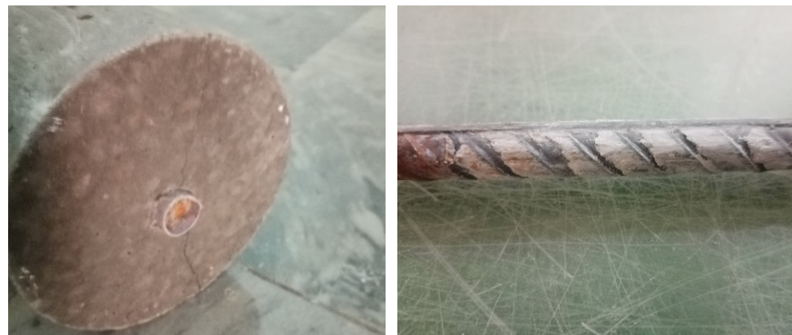
Figure 9. Yielding/bond failure in tested pull-out specimens.
