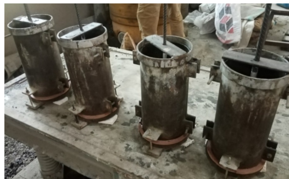
Figure 6. Cylindrical molds placed on a mechanical vibrating table before concrete pouring.
