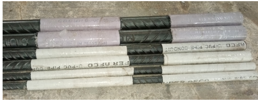
Figure 5. Steel bars enveloped with PVC tubes.
