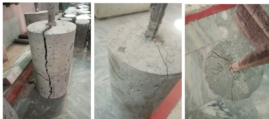
Figure 10. Splitting failure in pull-out test specimens.
