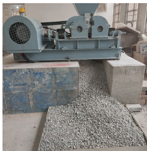
Figure 2. Concrete crusher machine.
