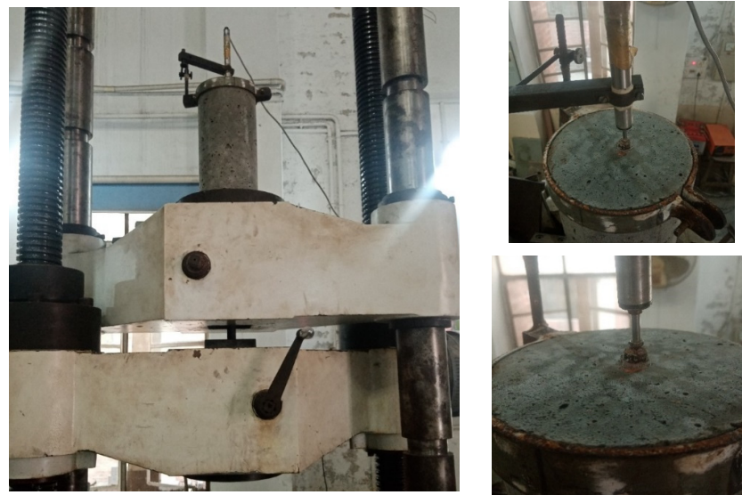
Figure 8. Pull-out test setup.
