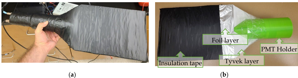
Figure 2. (a) Completed paddle detector; (b) Construction stages, showing the PMT holder, Tyvek, aluminum foil and insulating tape layers.
