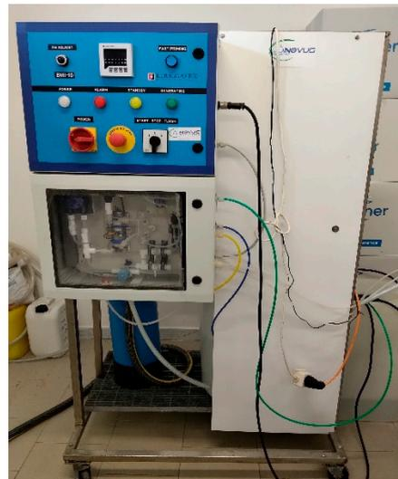
**Figure 1.** A prototype of an electrolytic generator used for the treatment of fruits and vegetables with electrolyzed water.
