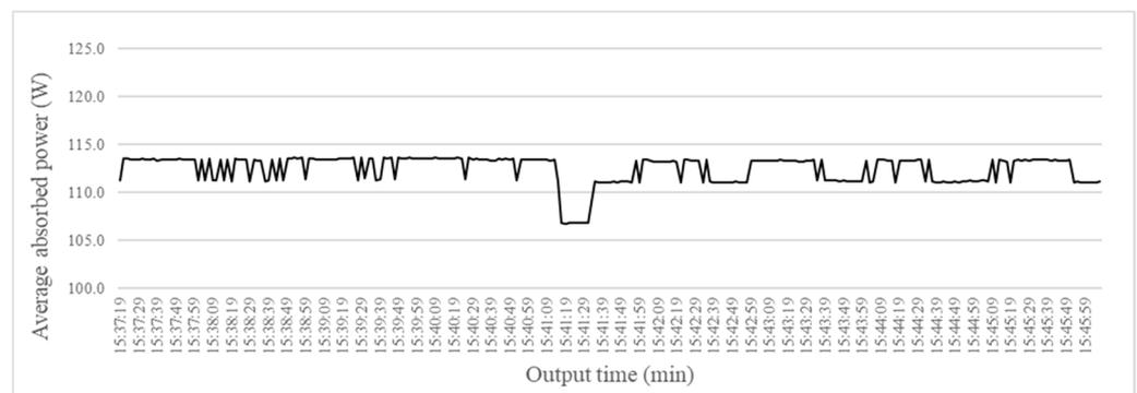
**Figure 9.** Global active electrical power absorption of the prototype EW generator, as a function of time.
