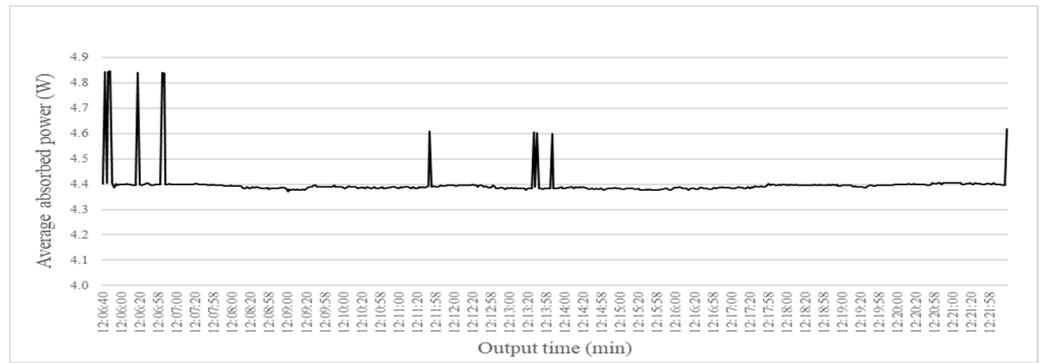
Figure 10. Active electrical power absorption of the main water pump.
