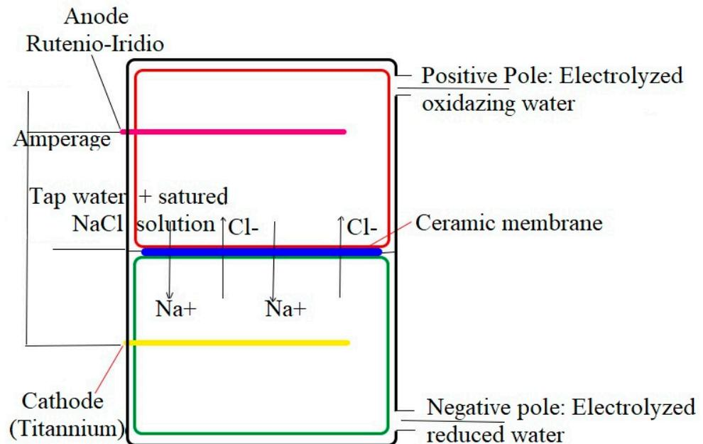
**Figure 3.** Schematic representation of the electrochemical activation process of saltwater [34].
