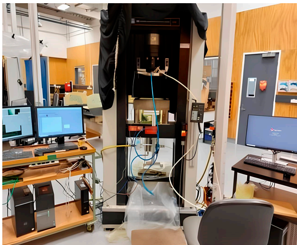
Figure 5. 2D radial flow experimental setup.
