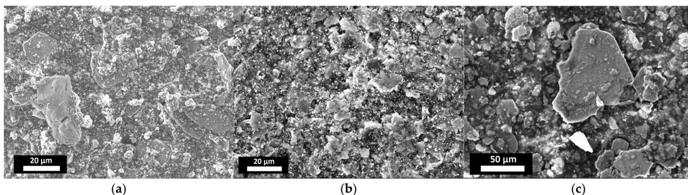
**Figure 1.** The SEM images of coatings: (a) sample 1002 (magnification  $\times 1000$ ), (b) sample 1006 ( $\times 1000$ ), (c) sample 1005 ( $\times 500$ ).
