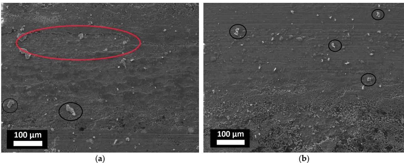
**Figure 8.** Surface of sample 1055 after testing under 10 N (a) and 23 N (b).
