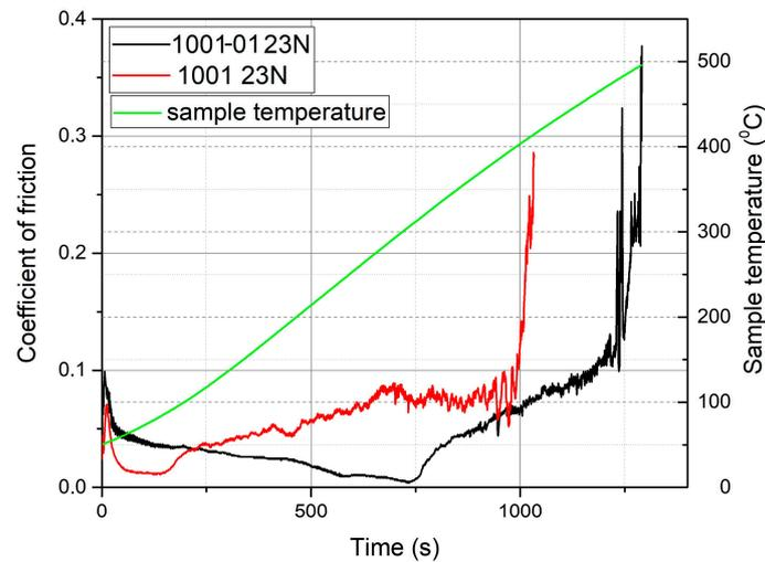
**Figure 5.** Changes in the coefficient of friction over time for samples 1001 and 1001-01 at a load of 23 N.
