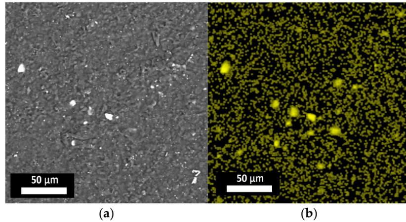
**Figure 2.** SEM image of the microstructure (a) and elemental mapping of sulfur (b) from the MoS<sub>2</sub> sprayed on sample 1002.
