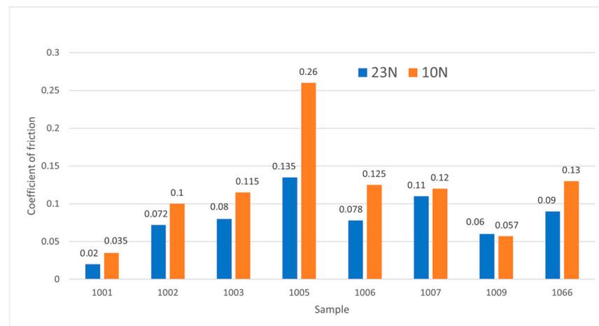
**Figure 3.** Results of measuring the coefficient of friction of coatings deposited on AISI 430 steel (group 1) at 150 °C.
