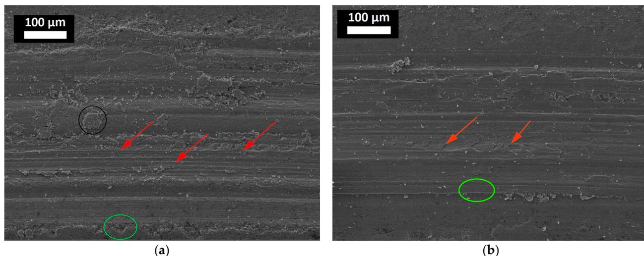
**Figure 6.** Surface of sample 1001 after testing under 10 N (a) and 23 N (b).
