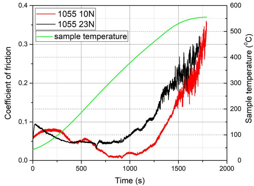
**Figure 7.** The change in the coefficient of friction over time for sample 1055 at loads of 10 N and 23 N.
