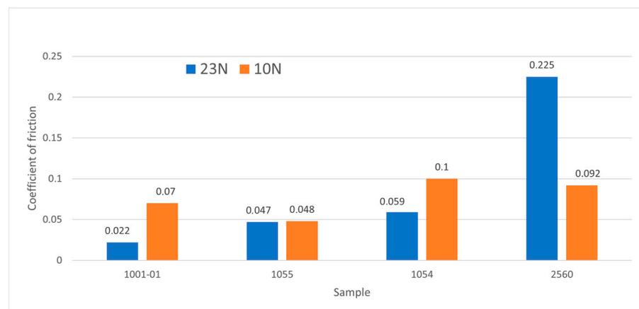
**Figure 4.** Results of measuring the coefficient of friction of coatings deposited on Inconel X-750 steel (group 2) at 150 °C.
