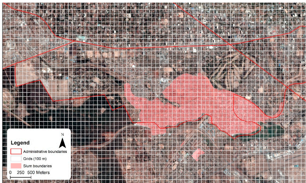
Figure 2. Gridded mapping frame to aggregate deprived areas, the example is showing Kibera slum in Nairobi (displayed on top of a PlanetScope image).
