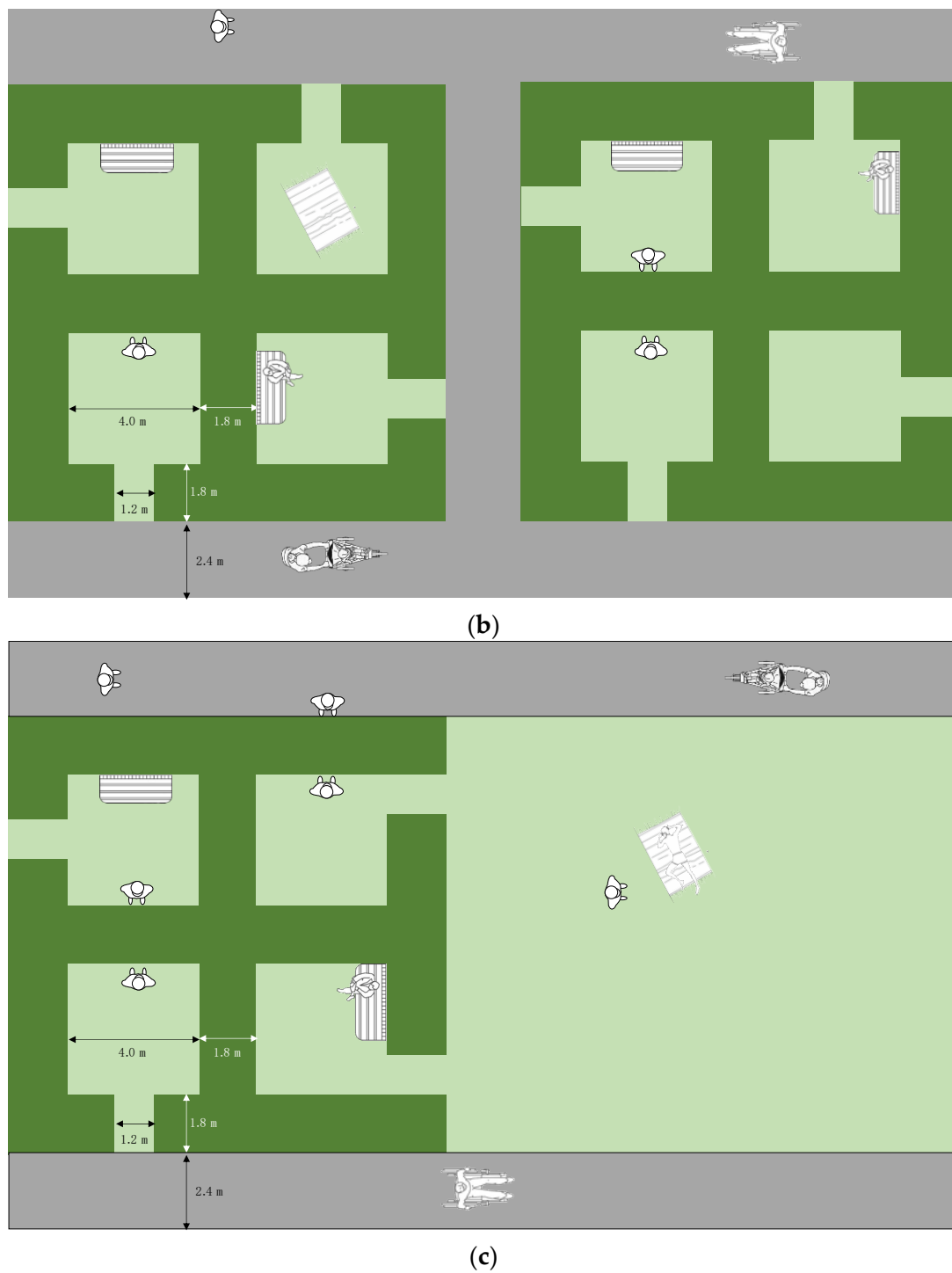
Figure 5. Design concepts for value-adding to pocket parks. (a) Design for narrow, sub-optimal green-spaces. (b) Compact design of 2 \times 2 spaces with intermediate communications pathway (c) Compact design of 2 \times 2 spaces adjacent to an open green space.
