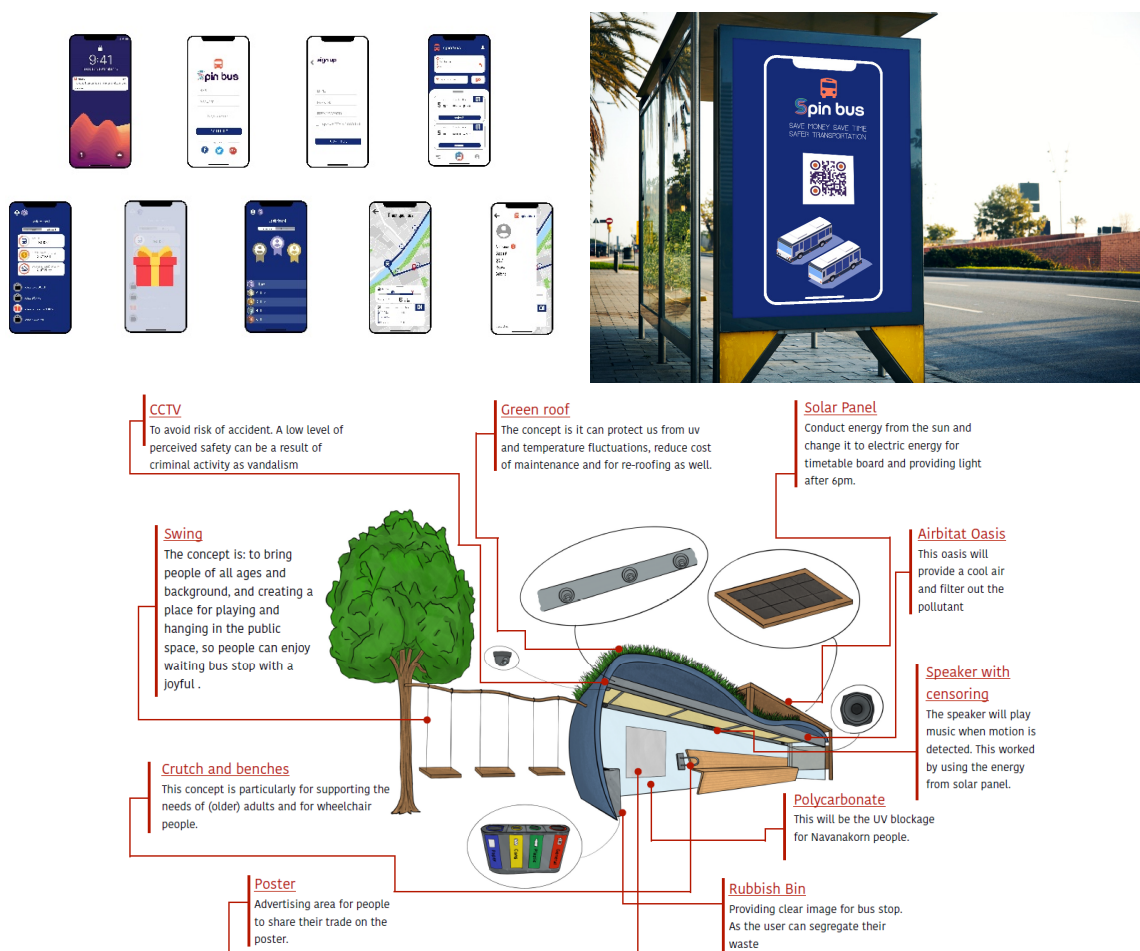
Figure 16. Spin Bus app with multiple windows (above, left) and integration of app with bus stop designs (above, right, and bottom). Graphics credits to Theerawan Junditthawong, Sajin Vimolpitayarat, Sakdithat Sapon, Parin Prakitsuwan, Satakamol Patcharatsathien, DBT244 class.
