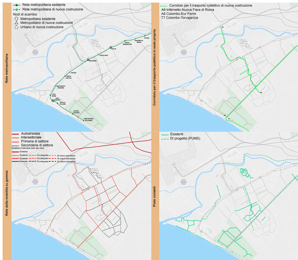
Figure 12. Rome Municipality X (Part), Local plan. System of infrastructures. Top left, underground network; top right, public transport corridors in their own premises; bottom left, road traffic; bottom right cycle-pedestrian paths (Source: elaborations by the students: S. Maiorano, F. J. Moran, A. Musto, C. Paloni, Urban Planning Laboratory of the Faculty of Architecture of Rome A.A. 2021–2022).
