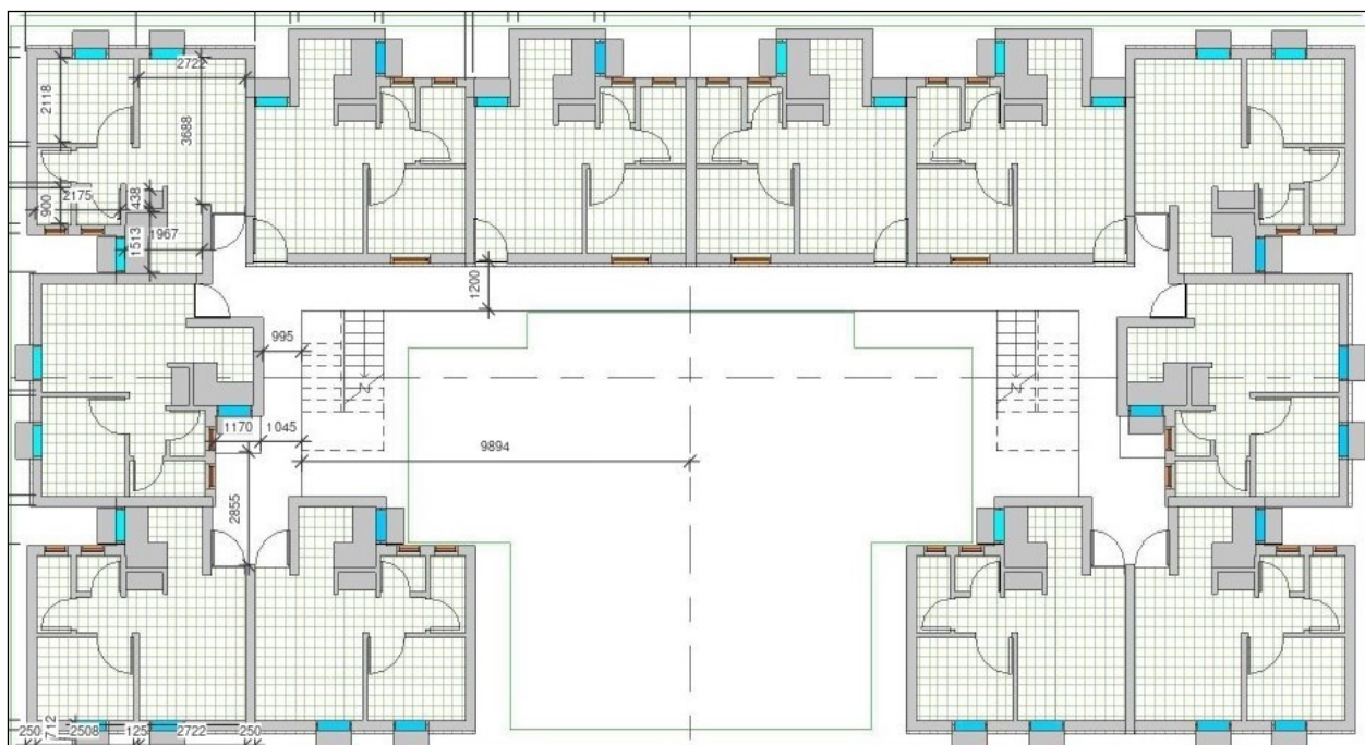
Figure 4. Illustration of an affordable housing cluster with 12 units on a floor. Source: MoHUA [15].
