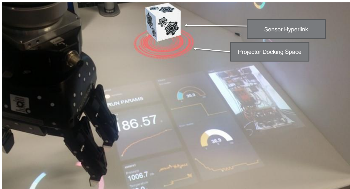
Figure 3. Representation of Hyperlinks in HoloLens (3D cubes) and projected surfaces (red circles).
