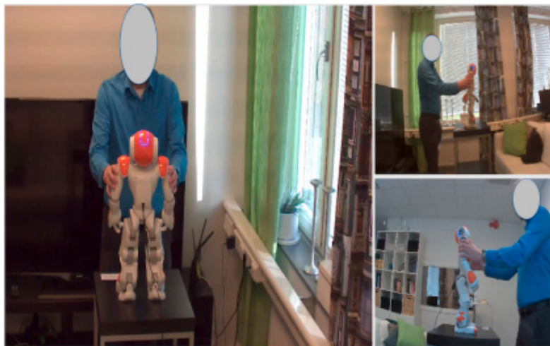
Figure 1. Experimental set-up where the participant interacts with the Nao in the Usability Lab. The participant interacts with the Nao by touching left and right arms to convey a particular emotion. Camera shots are supplied by the ELAN annotation tool: https://tla.mpi.nl/tools/tla-tools/elan/ .
