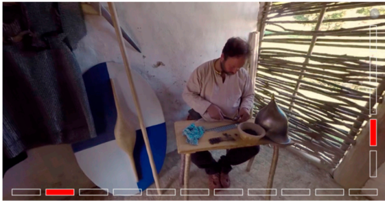
(a) The bar at the bottom shows if the PoI is to the right or left. The bar on the right shows if the PoI is higher or lower than the own viewing direction.
