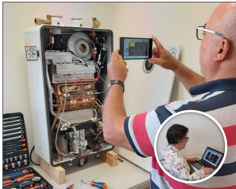
Figure 12. Remote team members collaborating through the AR-based tool: on-site participant being assisted by a remote expert.
